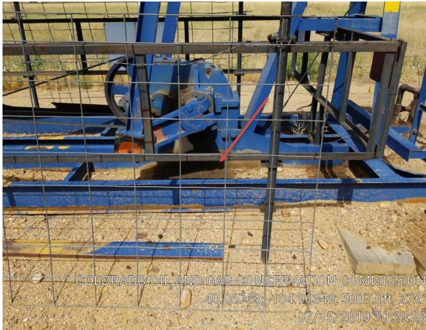
Pic 3 stained soil under pumping unit
