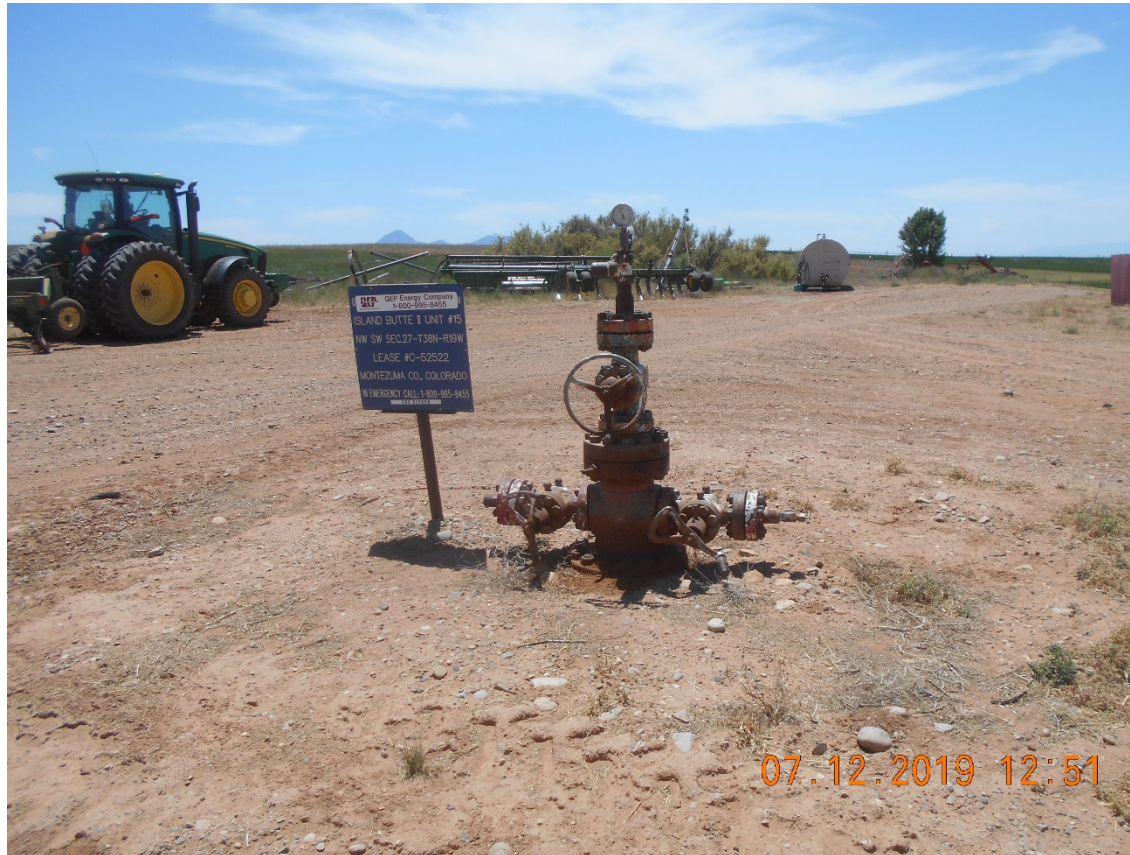
Injection Wellhead – Temporarily Abandoned
