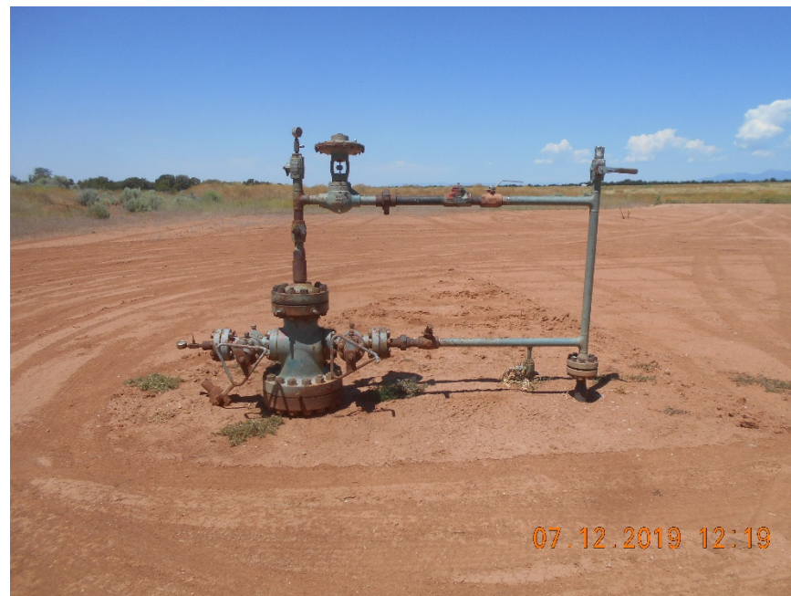
Injection wellhead.
