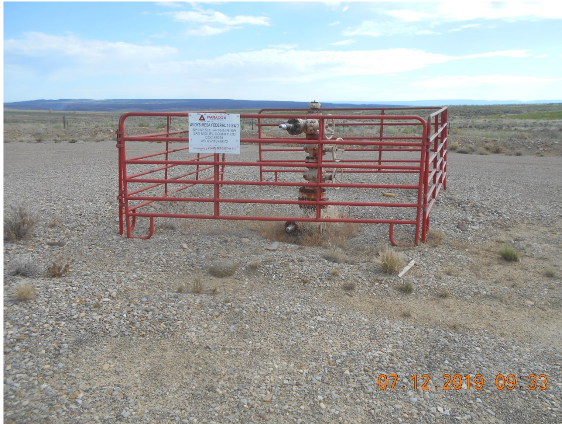
Injection Wellhead – Temporarily Abandoned
