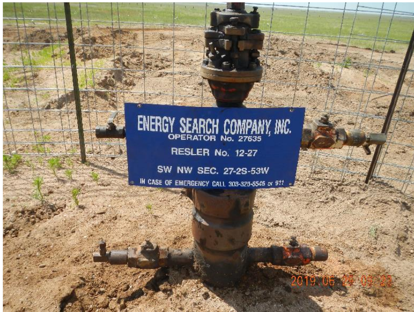
Photo 1: Wellhead with outlets plugged.
