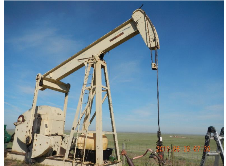
Photo 2: Disconnected bridgehead and pumping unit.
