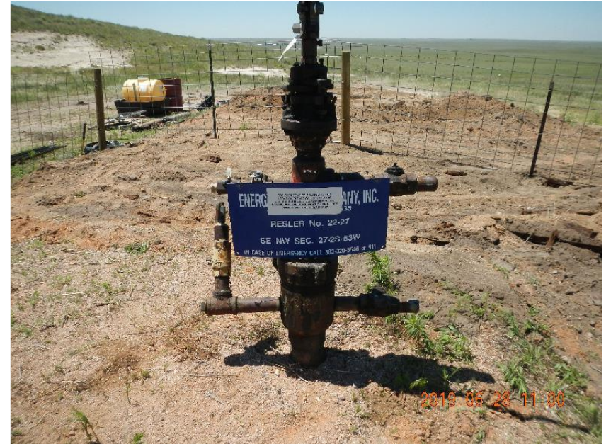
Photo 8: Wellhead with outlets bullpugged and well sign hung.
