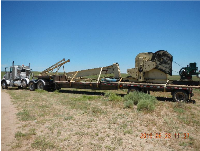
Photo 7: Pumping unit base and parts loaded on flatbed trailer for removal.
