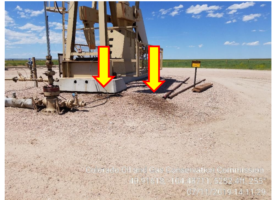
Photo 4 – Stained Soil at Wellhead
