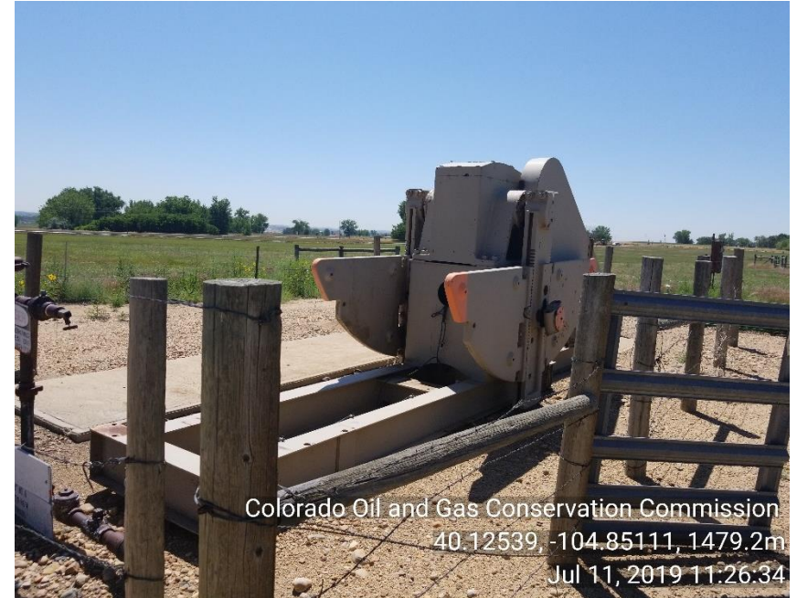
Photo 2 Unused equipment: PU base and gear box with weights.
