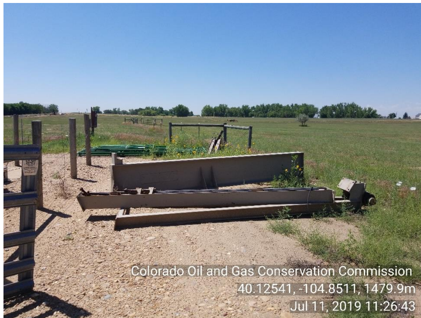
Photo 3 Unused equipment: Walking beam, pitman arms, horses head and cattle panels.
