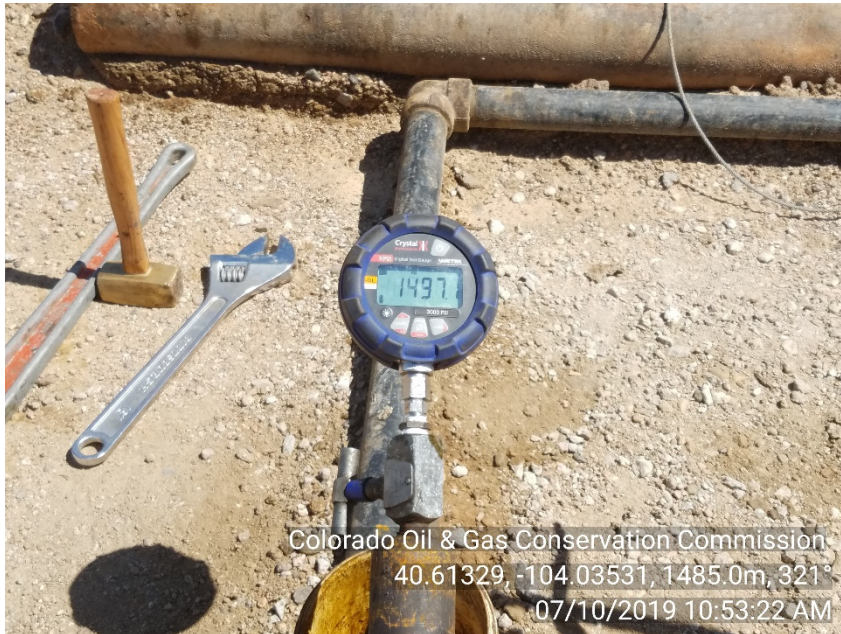
Photo #7 State 36-16 Injection Well Shut-In | SI 10-min reading | UIC - MIT Csg. Press: 1497#
