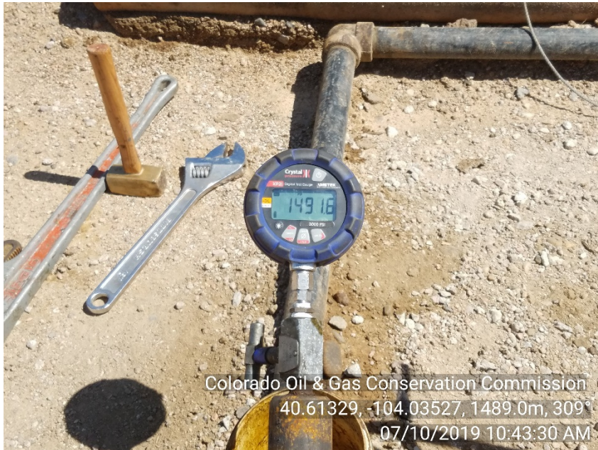
Photo #5 State 36-16 Injection Well Shut-In | SI Start Test | UIC – MIT 15 min after pressure up to stabilize Csg. Press: 1492#
