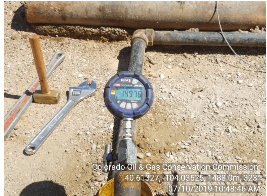
Photo #6 State 36-16 Injection Well Shut-In | SI 5-min reading | UIC - MIT Csg. Press: 1498#
