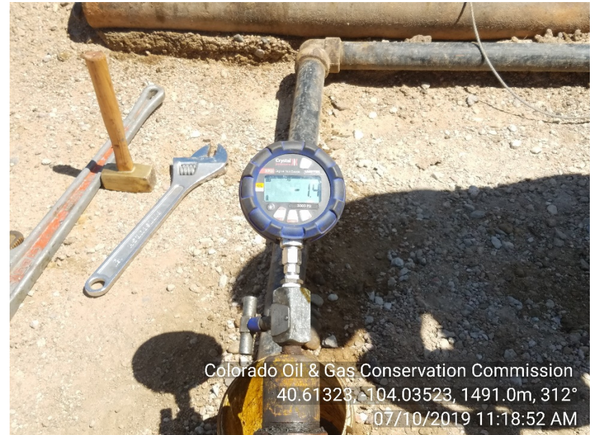
Photo #10 State 36-16 Injection Well Shut-In | SI Post Test , bled down | UIC - MIT Csg. Press: 0#
