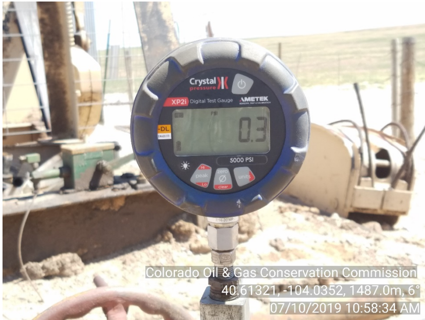
Photo #9 State 36-16 Injection Well Shut-In | SI End Test | UIC - MIT Tbg. Press: 0#
