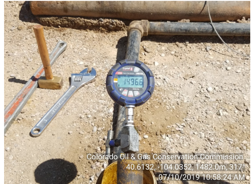
Photo #8 State 36-16 Injection Well Shut-In | SI 15-min reading, End Test | UIC - MIT Csg. Press: 1498#
