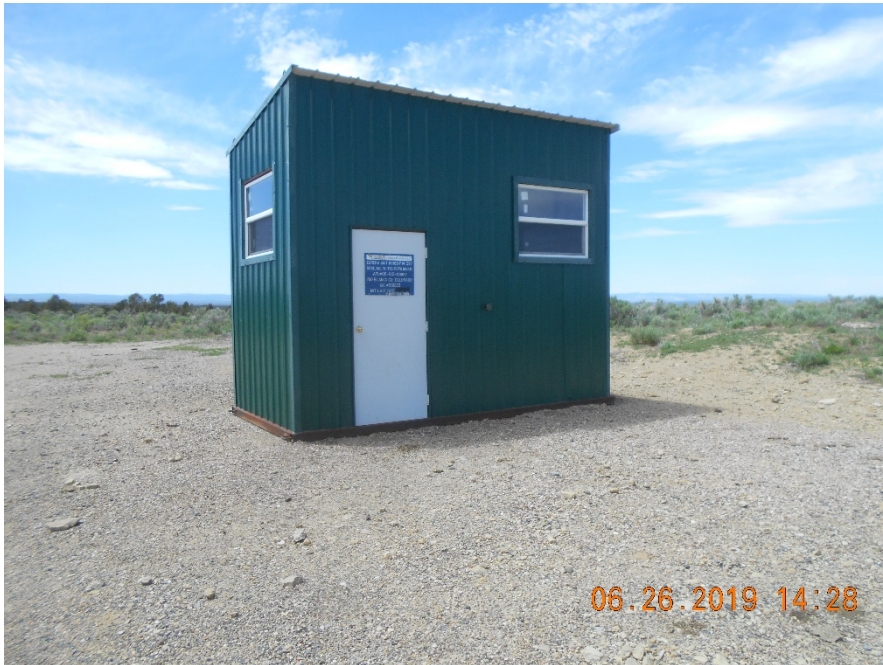
Injection wellhead housing
