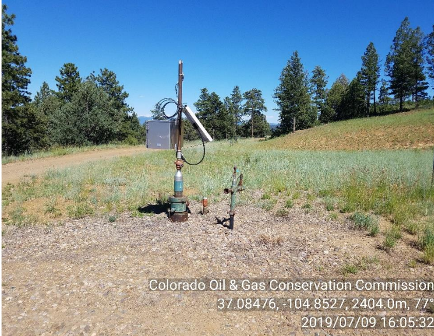
PHOTO 1: WELLHEAD/ UNUSED EQUIPMENT (TWO 2" AND ONE 1" RISER). REMOVE UNUSED RISER'S IN ACCORDANCE WITH NTO & RULE 603.f. CA DATE 10/9/19
