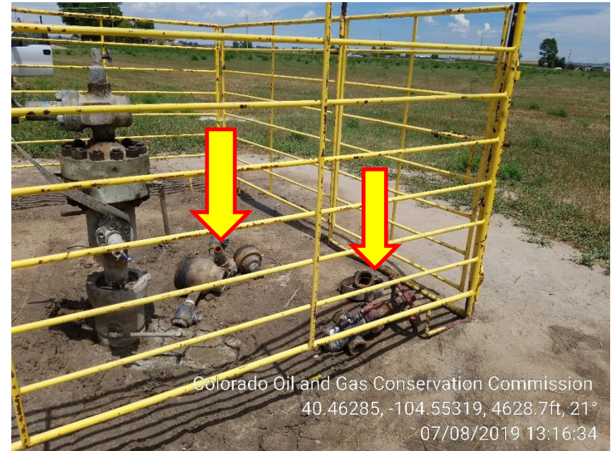
Photo 4 – Unused Wellhead parts
