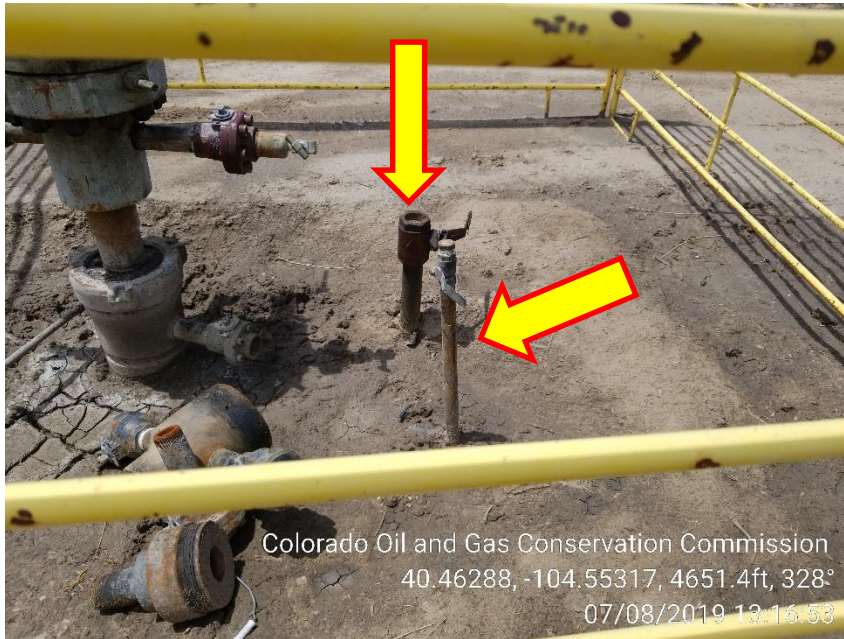
Photo 5 – Unmarked 1” and 2” Risers
