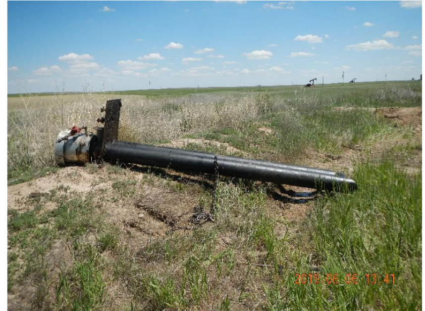
Photo 2: Removed flame tube laid down.
