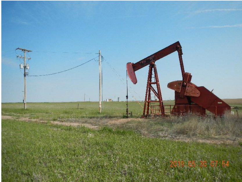
Photo 1: Oliver Warren pumping unit and power lines coming into location.
