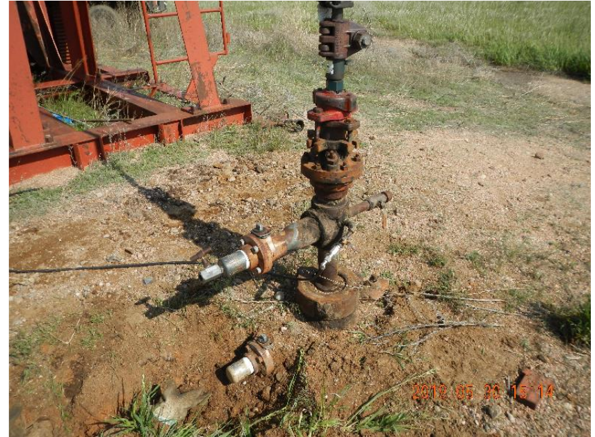
Photo 20: Wellhead with outlets bull plugged.
