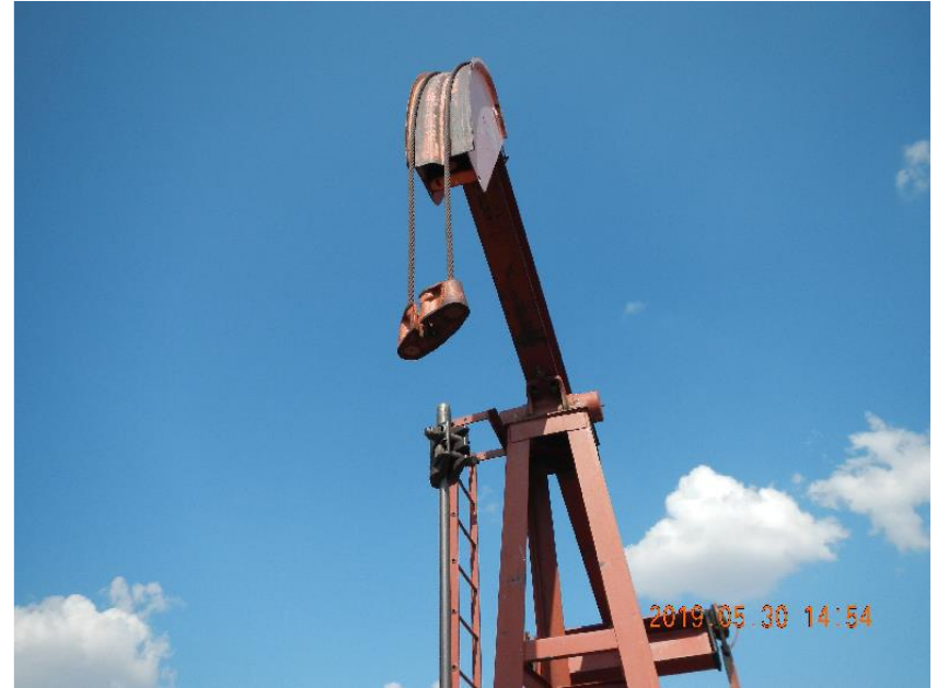
Photo 18: Disconnected bridle from wellhead.
