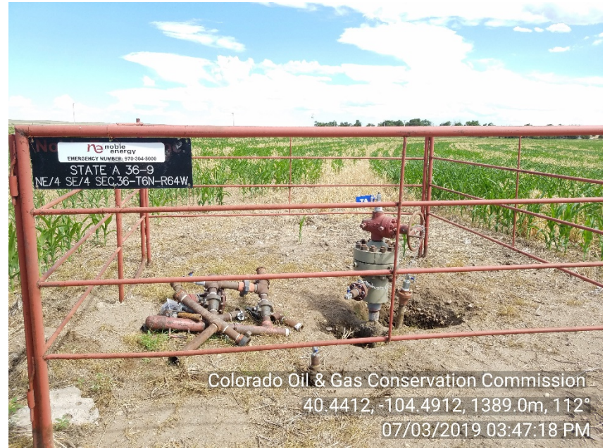
Photo #2 State A 36-9 Wellsite Temporarily Abandoned | TA Correct Emergency number NOW posted New Current MIT
