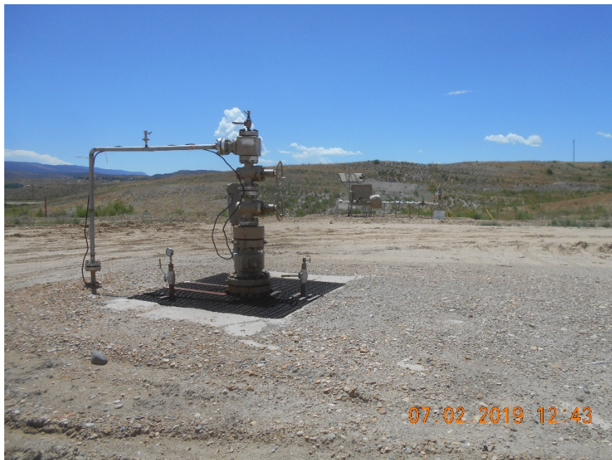
Injection wellhead
