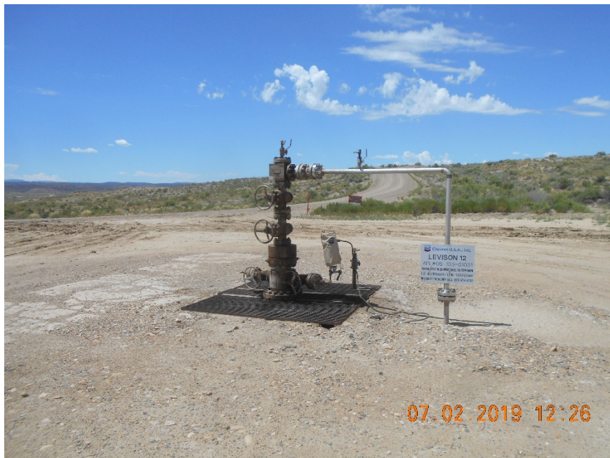
Injection wellhead
