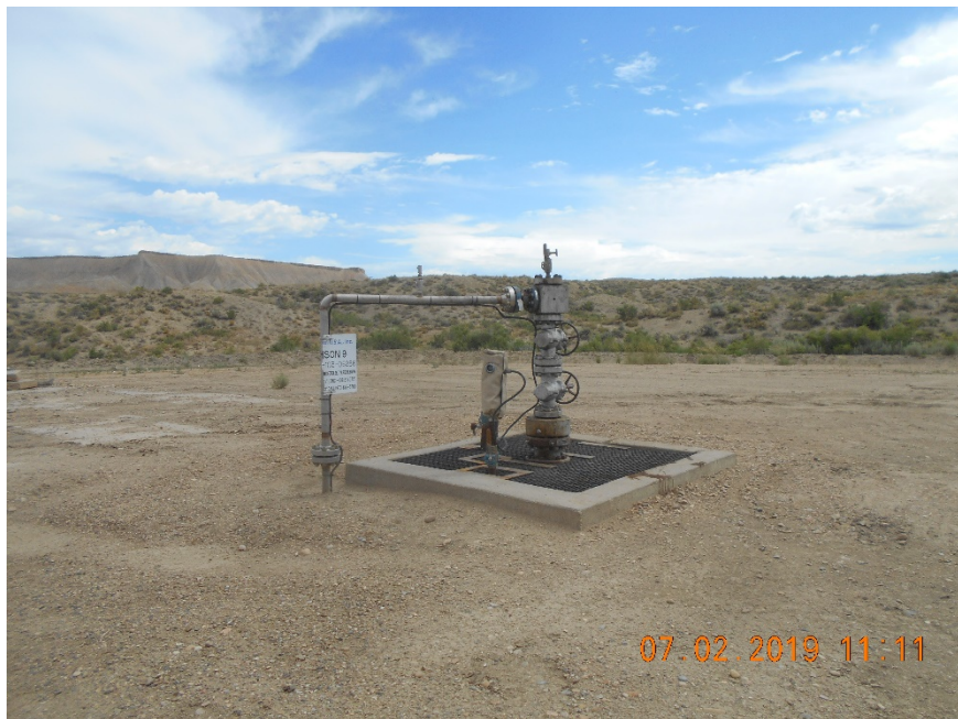
Injection wellhead
