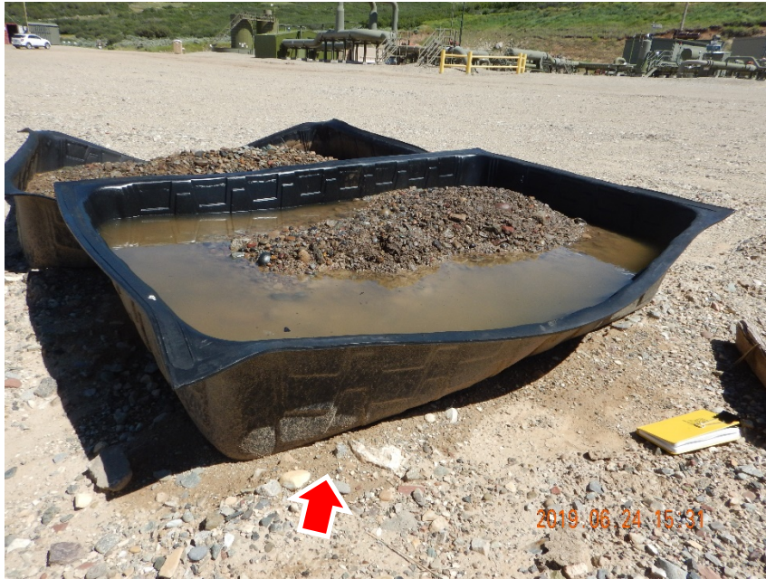
Photo #11 – Unidentified stockpile of impacted soil located at northwest corner of location. Stockpiles contained precipitation with little freeboard (~1"). Stained and saturated soil beneath storage containers indicate that fluids have escaped containment previously (red arrows).
