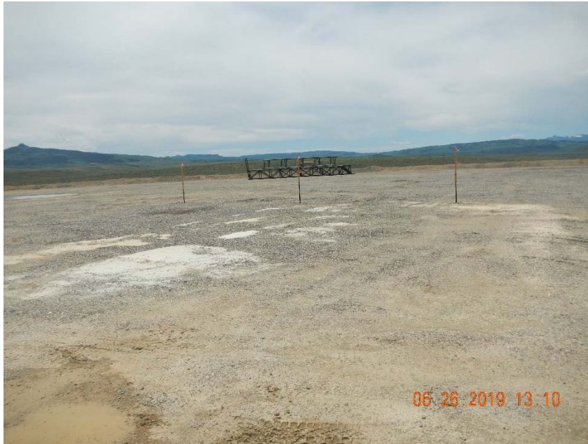
Photo 13. Frack sand spilled on location.
