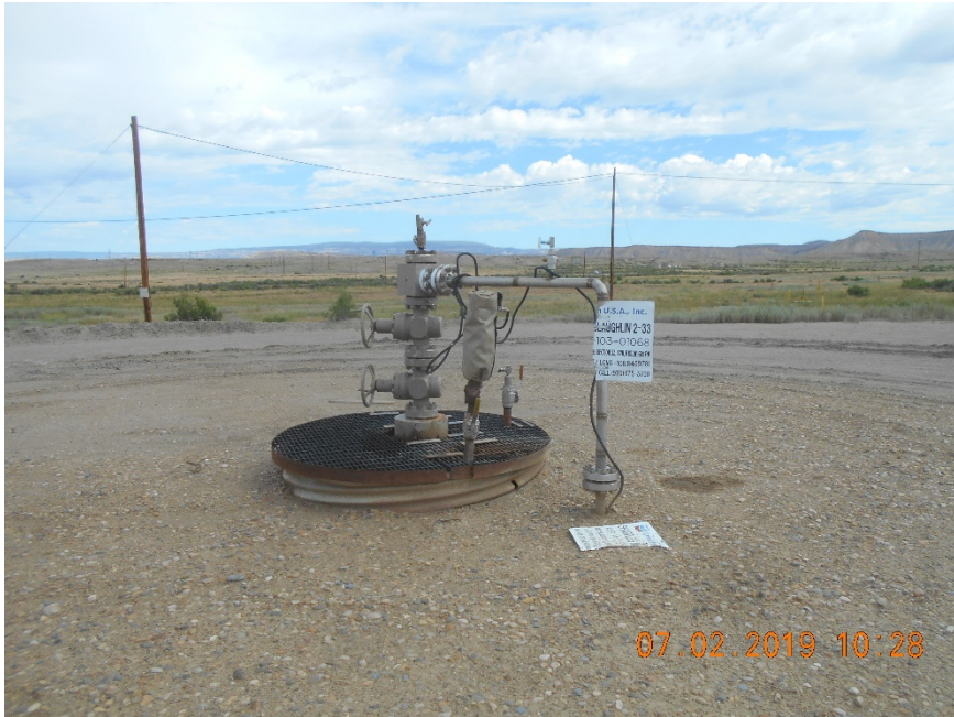
Injection wellhead
