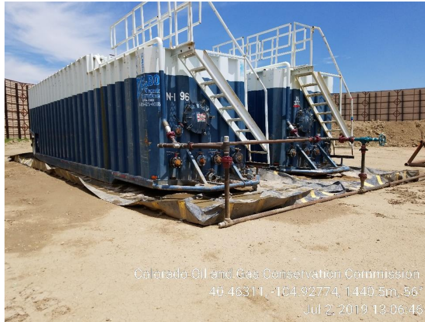
Photo 1: No grounding rod
