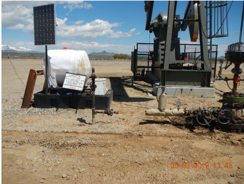
Photo 3. Stained soil at wellhead, chemical containment full of stormwater.
