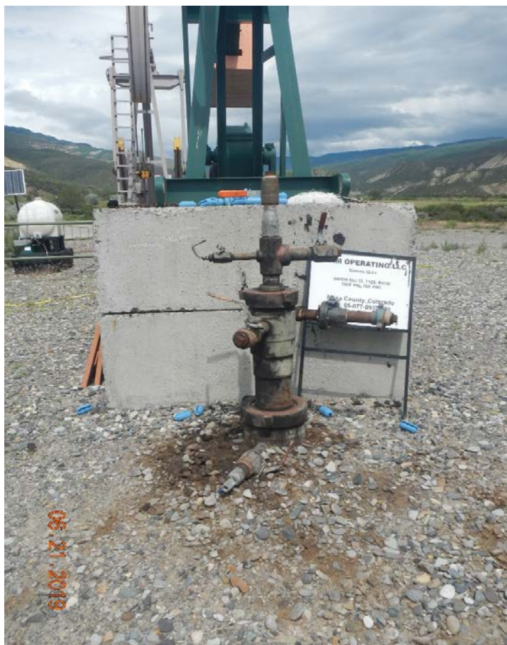
Photo#2: Localized area of stained soil at well head area.
