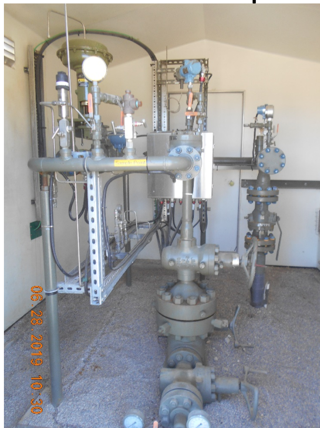
Injection wellhead inside housing
