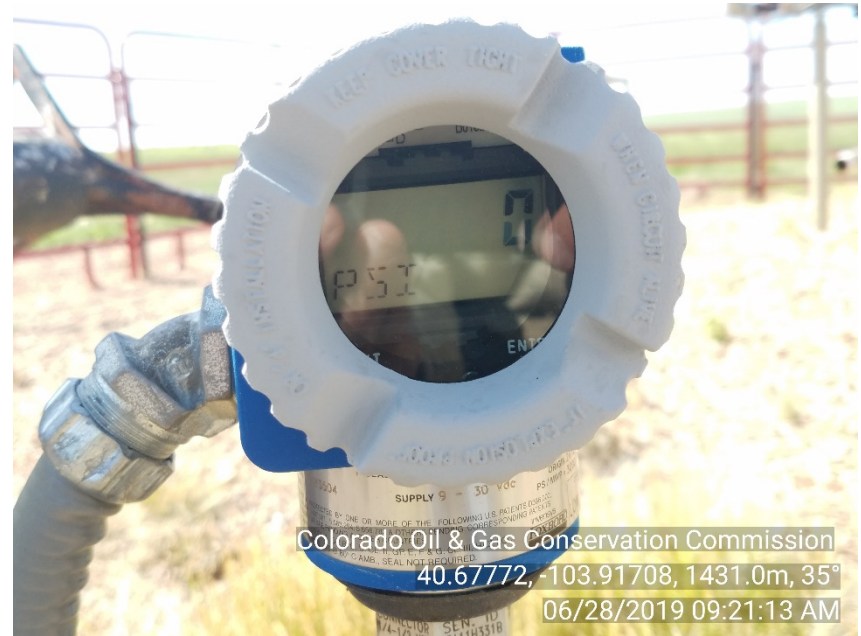
Photo #4 Lilli Unit 8-12 UIC - Injection Well Csg Press: 0# Shut-In | SI Not Injecting
