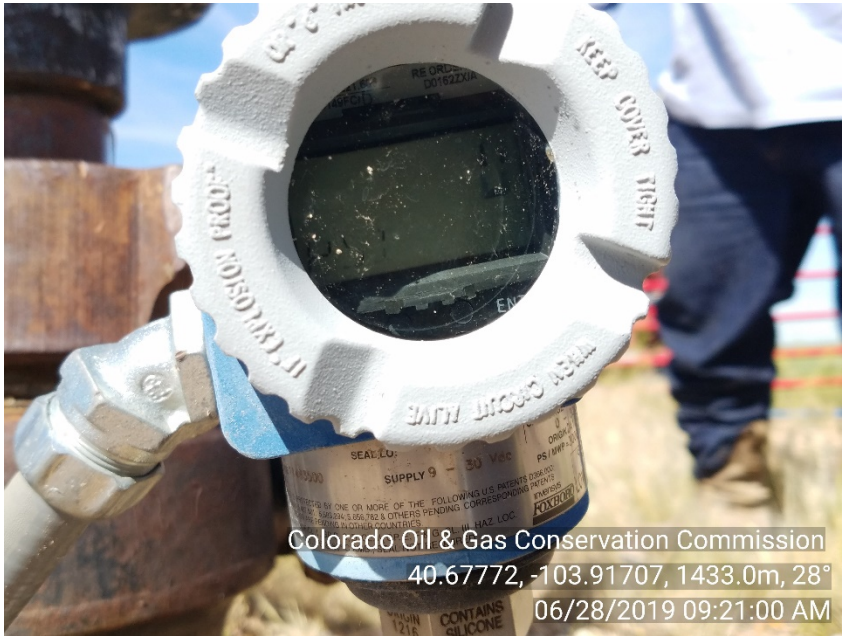
Photo #5 Lilli Unit 8-12 UIC - Injection Well Bradenhead Press: 0# Shut-In | SI Not Injecting
