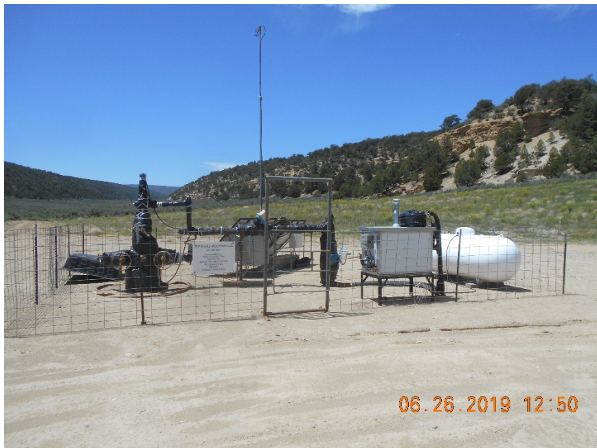
Injection wellhead & line heater
