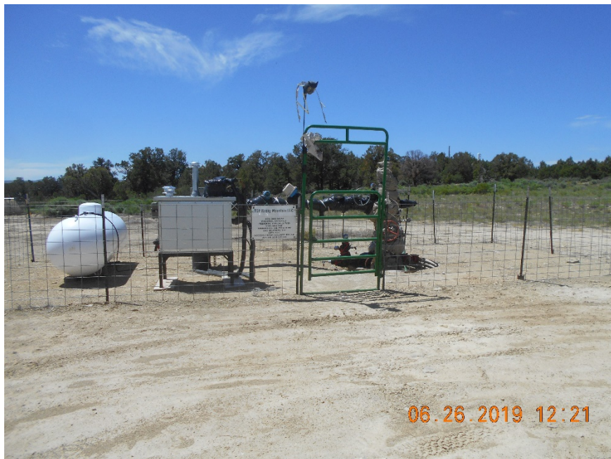
Injection wellhead & line heater
