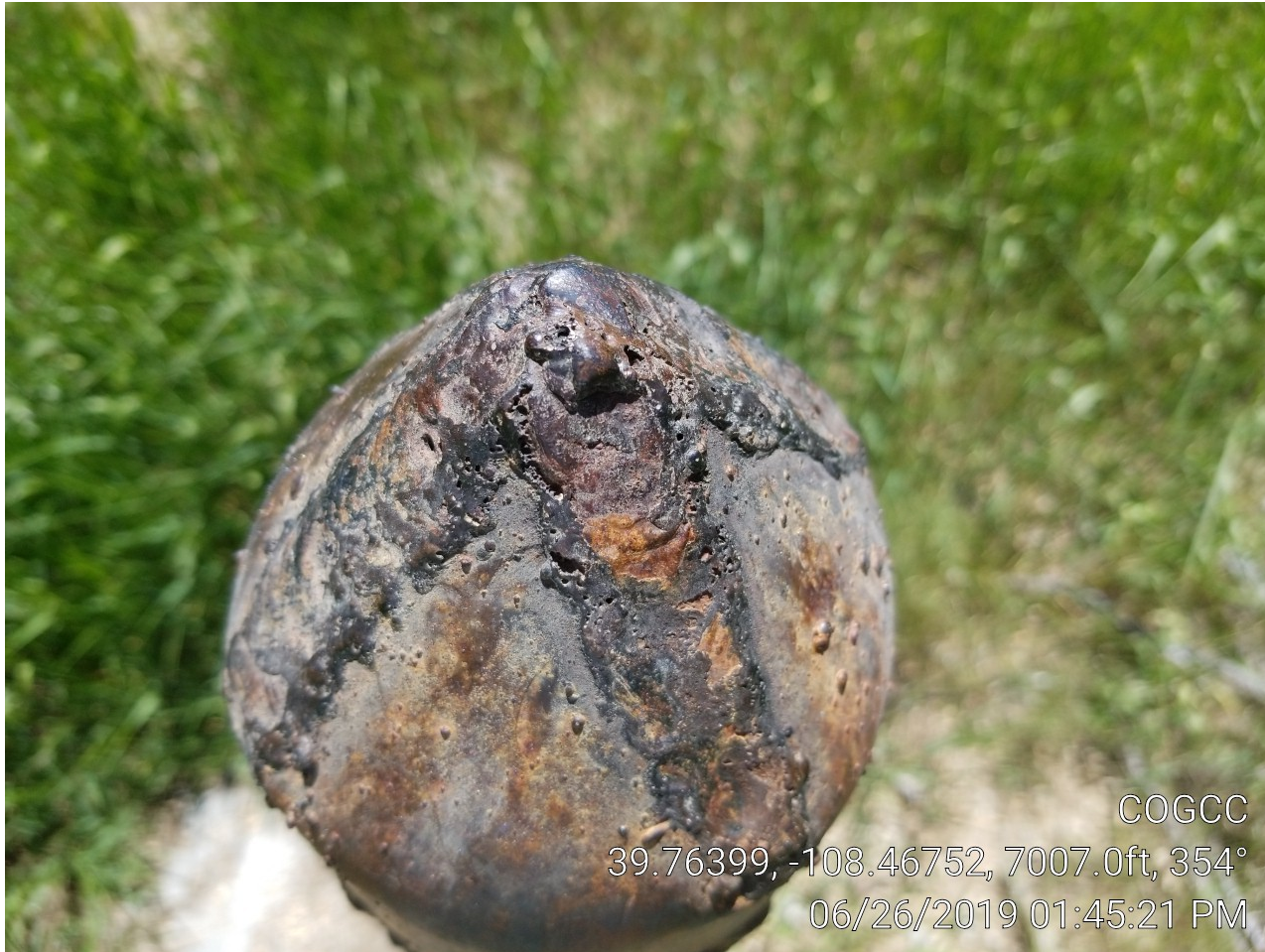
Photo 2. Top of P&A marker with several pin holes in welds venting gas.
