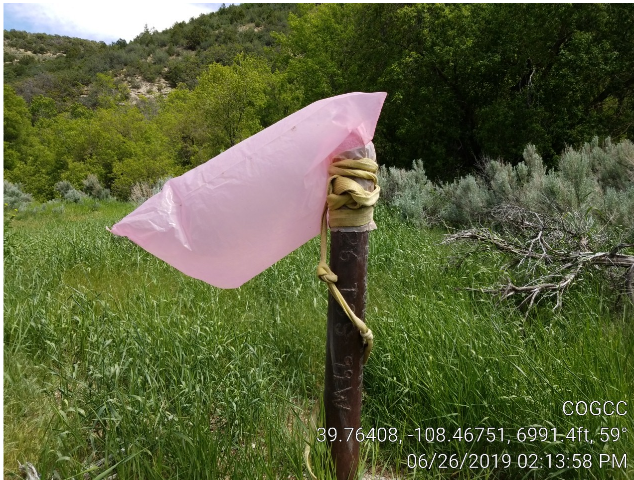
Photo 3. Gas filled bag on well head.
