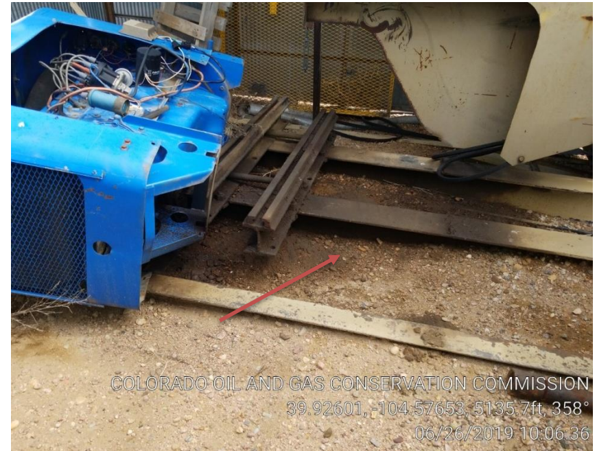
Pic 4 stained soil inside motor house of pumping unit
