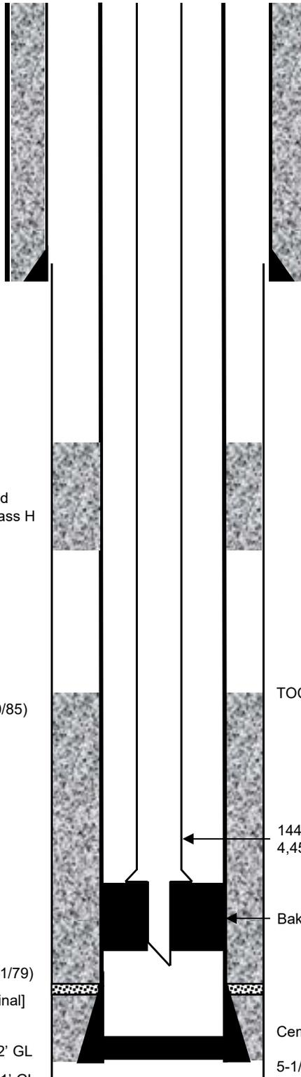
Cemented surface casing w/ 400 sx Pozmix A with 2% gel and 1/4# flocele/sx, tailed with 100 sx common cement w/2% CaCl. Found TOC 22' below RKB. Spotted with 50 sx common cement with 2% CaCl.
