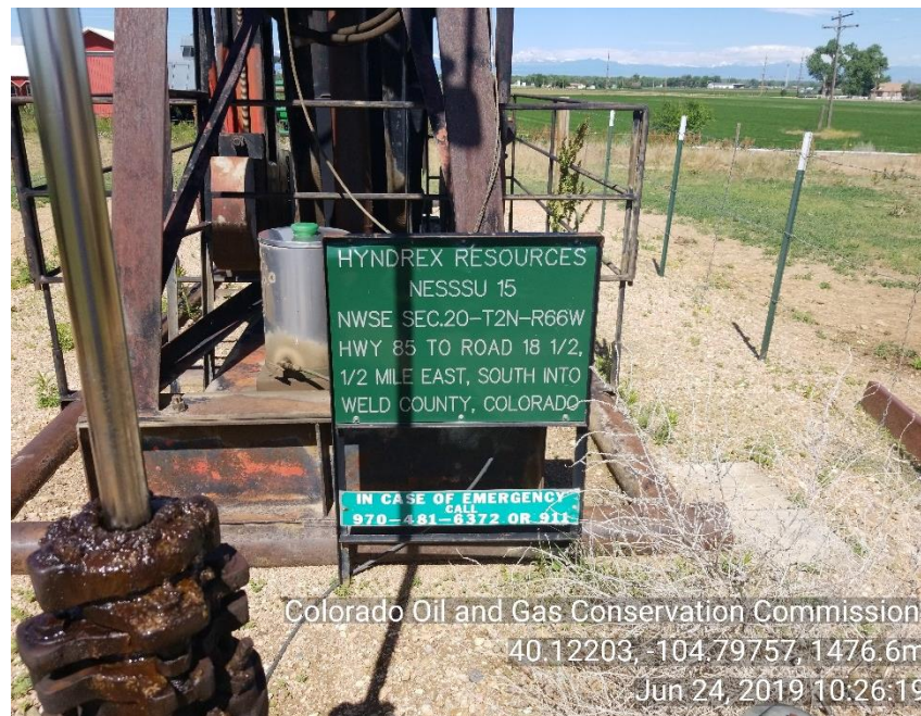
Photo 2 WH sign does not reflect current operator and emergency contact number.
