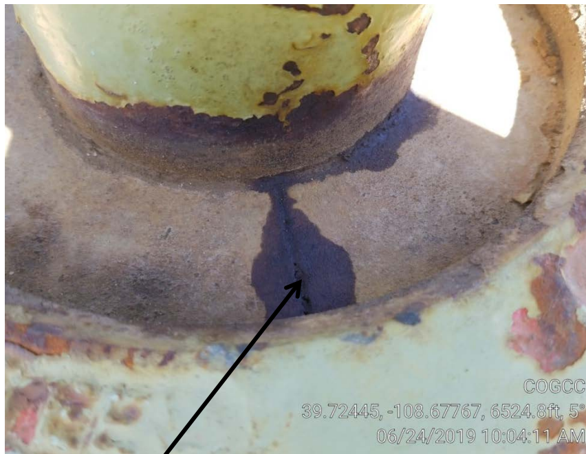
Photo 2. Gas leak at well head.
