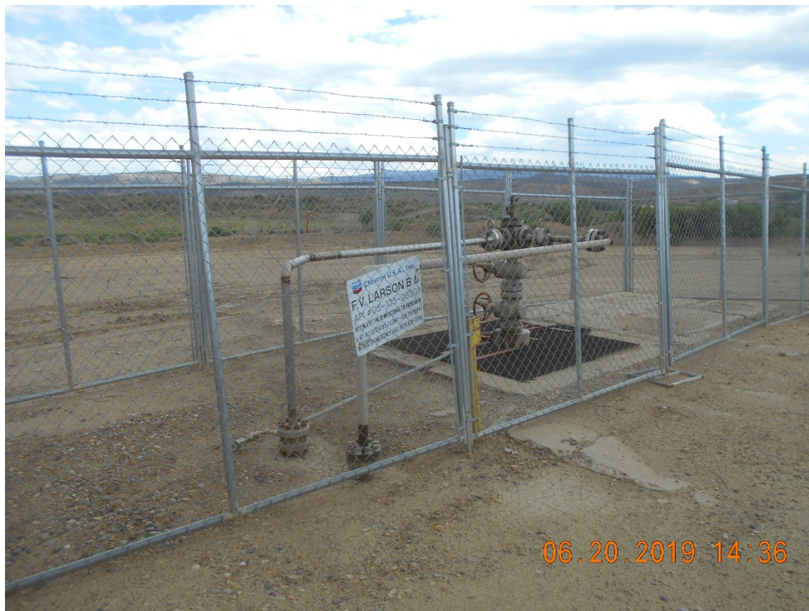
Injection wellhead
