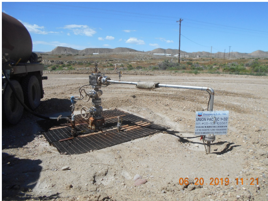
Injection wellhead
