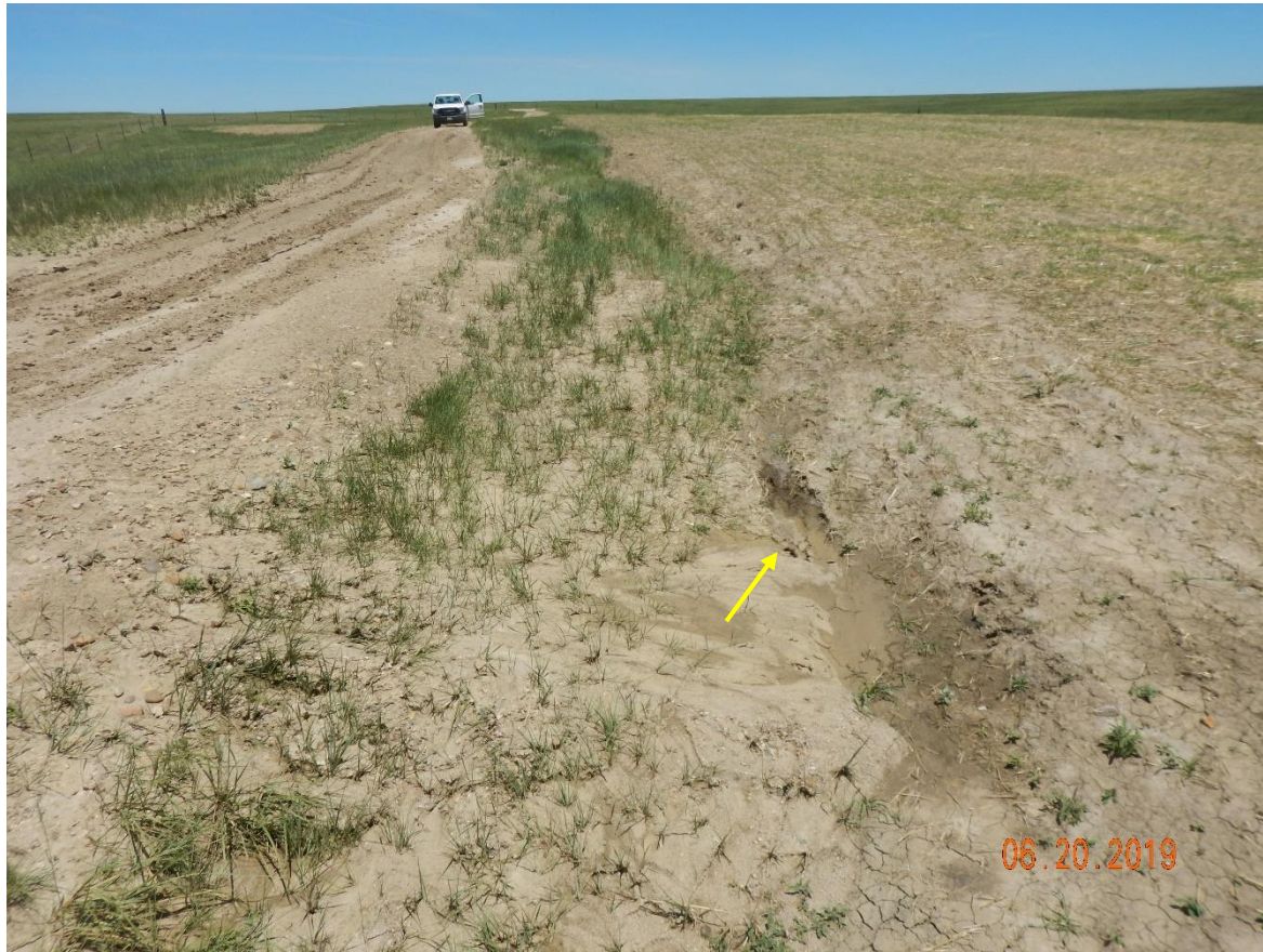
Photo 5: Photo taken from the southwest end of the location, facing northeast. Photo shows stormwater runoff is beginning to cause erosion degradation with sediment discharge onto the adjacent lands. Advise installing BMPs
