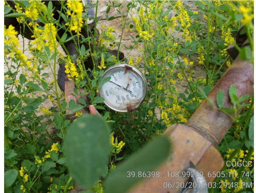
Photo 15. Tubing gage @ 0 psi.
