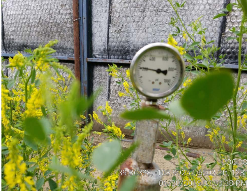
Photo 14. Casing gage @ 200 psi.
