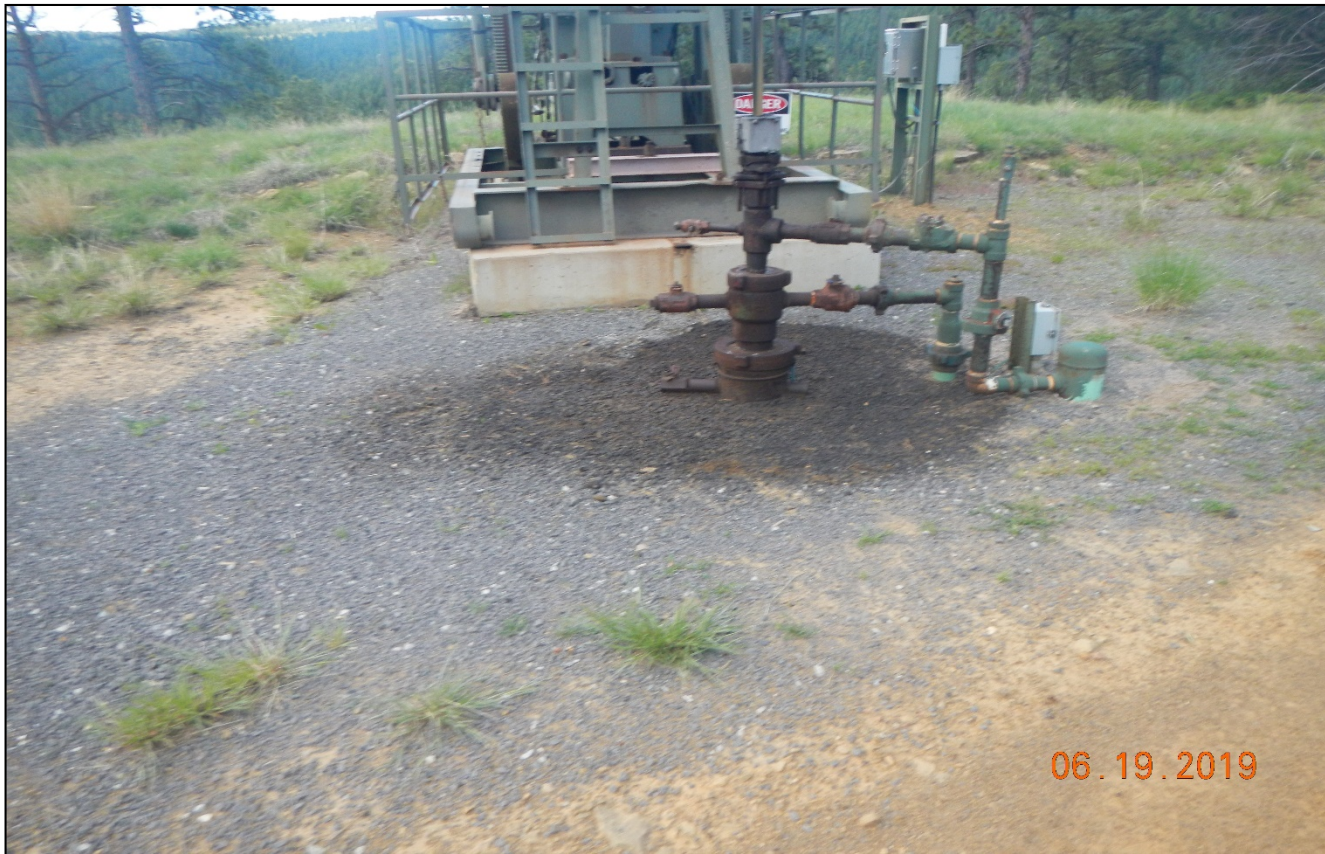
Photo 2. There is dark stained soil around the wellhead.
