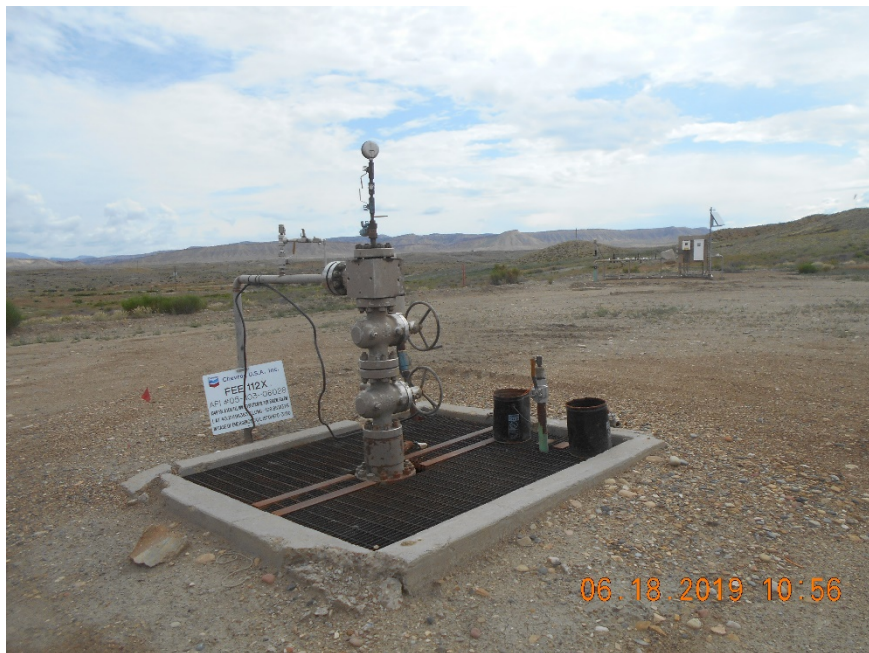
Injection wellhead. Trash buckets on cellar grate.
