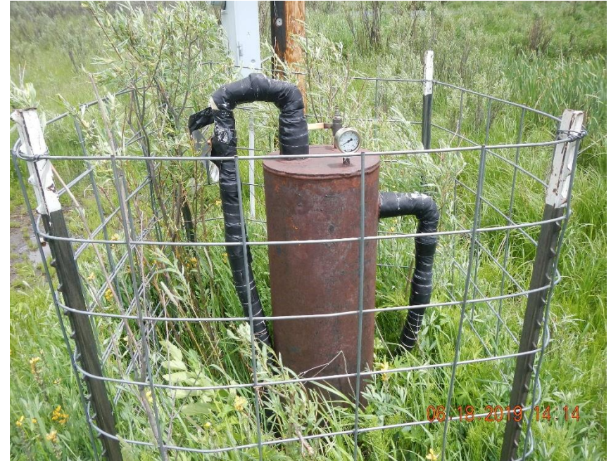
Drop out tank with 8 psi on pressure gauge.
