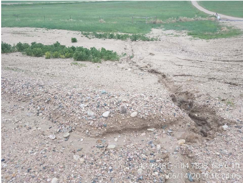
Photo 3 – Rill developing around site berm where access road enters pad on south side of pad.
