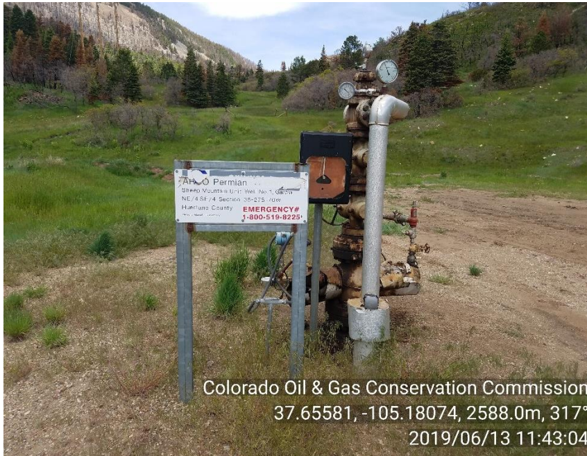
PHOTO 1: WELLHEAD/ WELLSIGN/ CURRENT OPERATOR IS NOT POSTED ON WELLSIGN 911 IS NOT POSTED AS EMERGENCY CONTACT. IF 911 SERVICES THIS AREA POST 911 AS EMERGENCY CONTACT ALSO POST CURRENT OPERATOR SIGN IN ACCORDANCE WITH 210 SERIES RULES. CA DATE 7/13/19.
