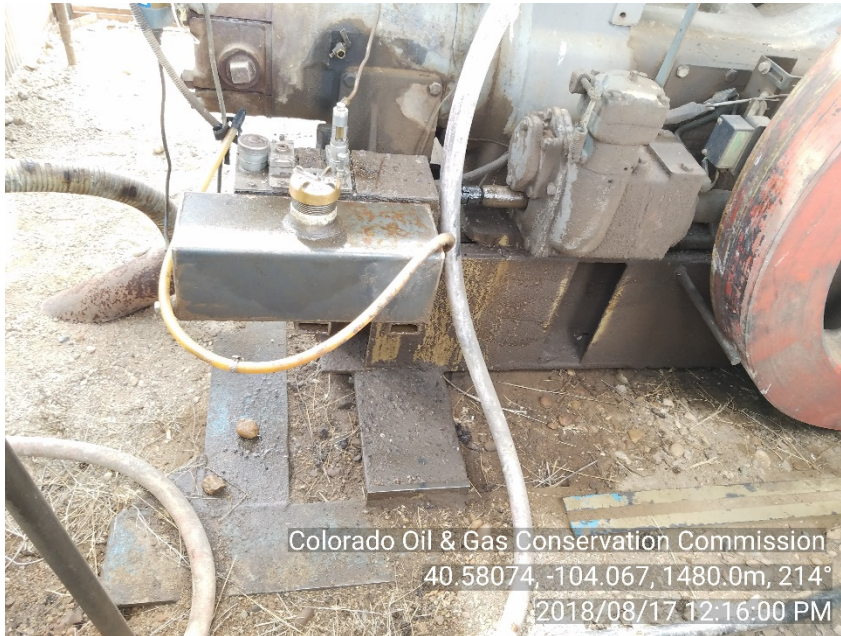
Photo #5 Dryer #1 Engine house Stained soil near engine base from prior insp.
