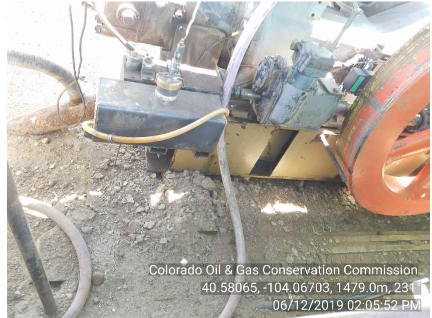
Photo #6 Dryer #1 Engine house Stained soil near engine base – Appears mitigated
