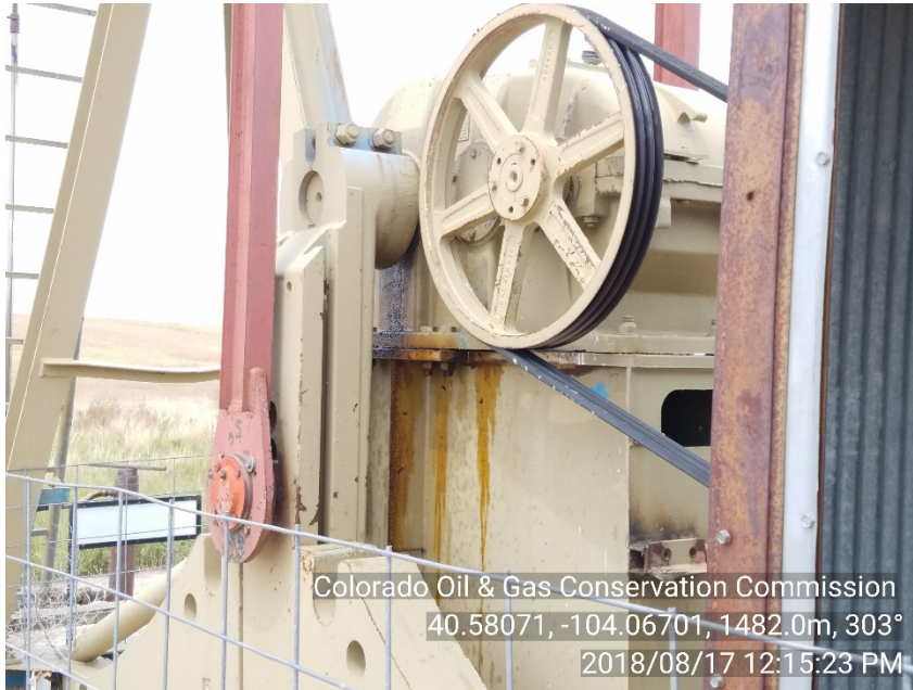
Photo #7 Dryer #1 Pumpjack Gearbox stain & apparent seepage from prior insp.
