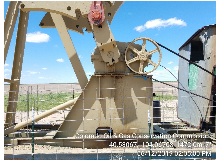
Photo #8 Dryer #1 Pumpjack Gearbox stain & apparent seepage Appears mitigated
