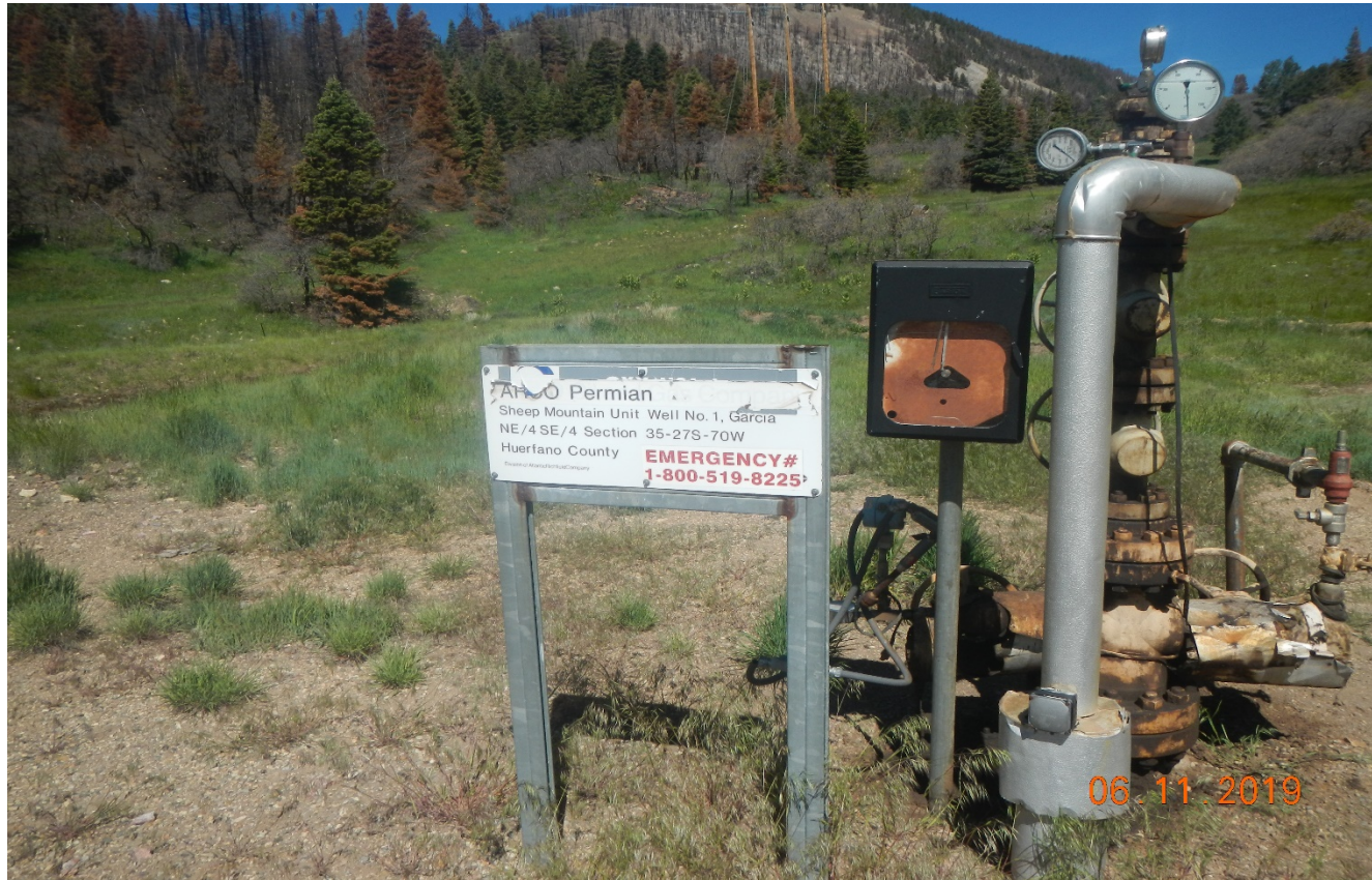
Photo 1. The operator name on well sign is not legible.
