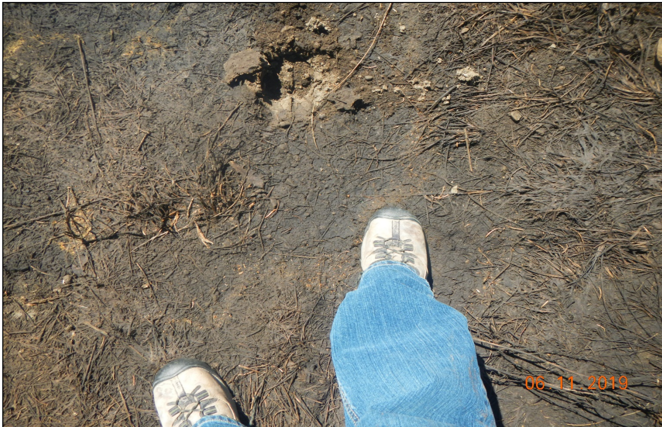
Photo 3. View of stained soil with strong hydrocarbon odor.
