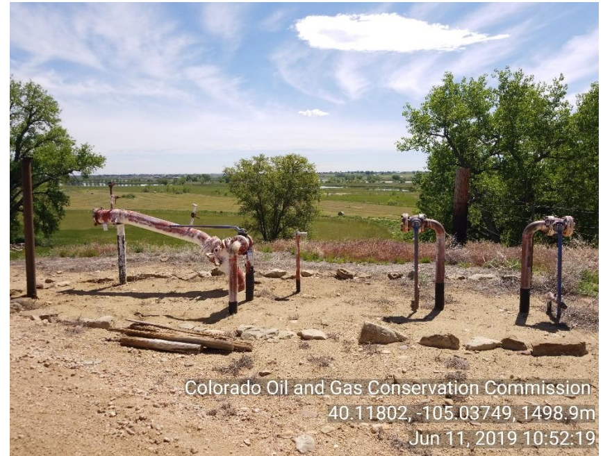
Photo 2 Pig launcher.
