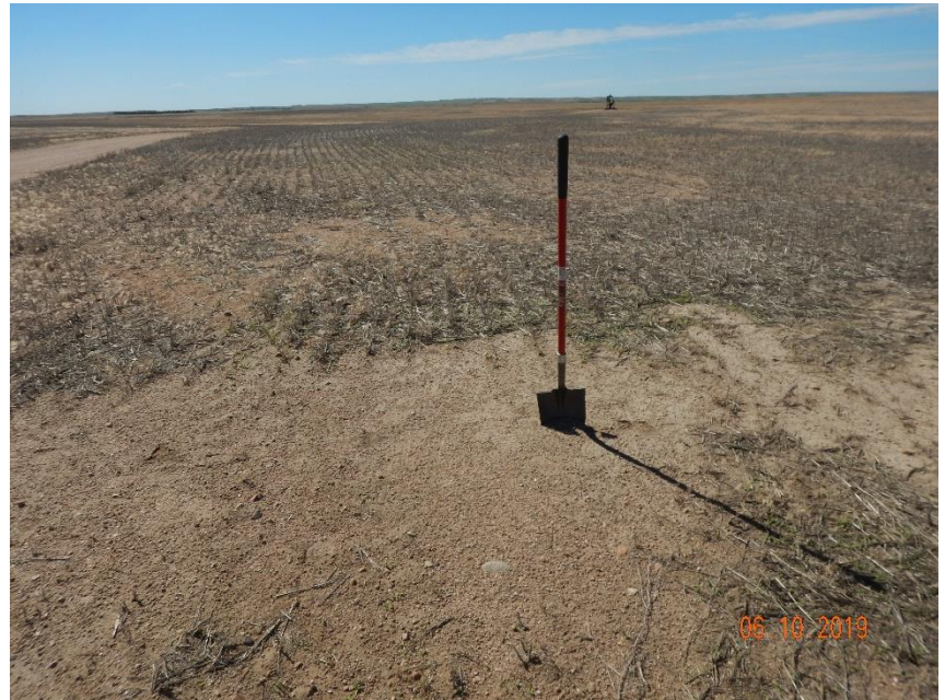
Photo 2: Photo taken from well location, facing west. Photo shows inspector was only able to easily penetrate the top few inches of soil on the location. Compaction concerns may exist.
