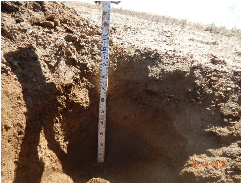
Photo 3: Photo shows inspector dug a compaction test pit. Photo shows possible compaction zone.
