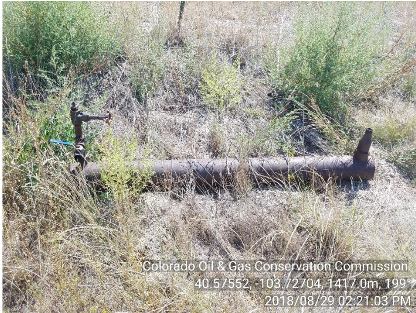
Photo #9 Northrup 1-14 Unused Equipment Unused volume pot from prior insp.
