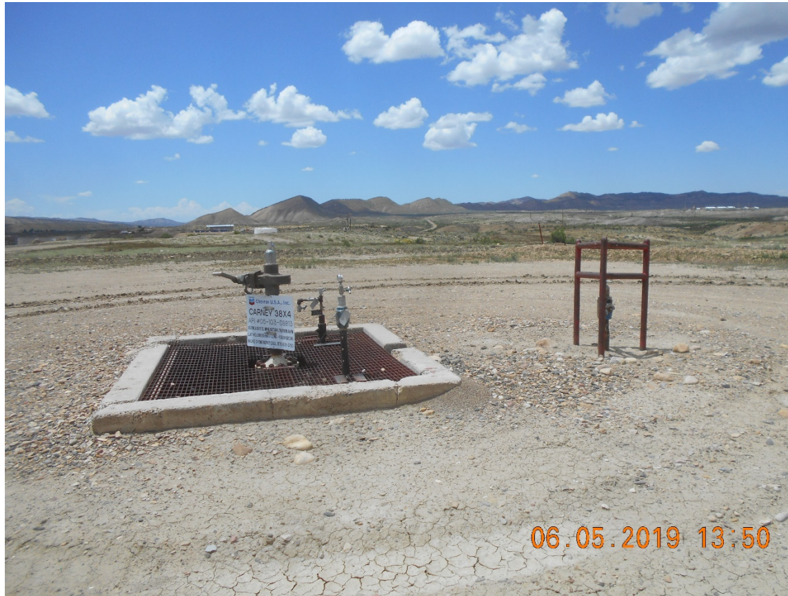
Injection wellhead
