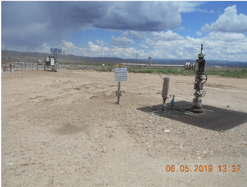
Injection wellhead
