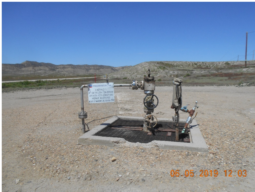
Injection wellhead
